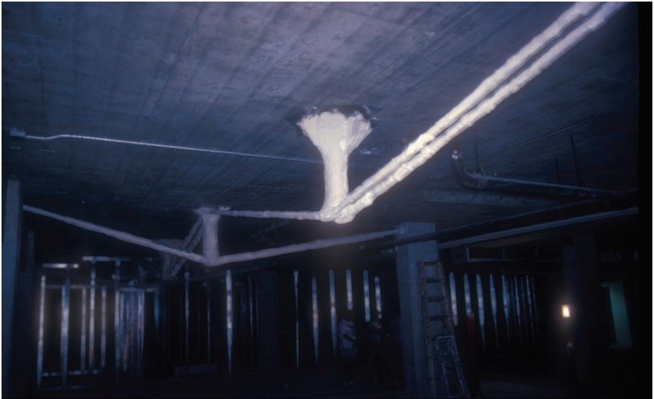
Fig. 10 – Two-Way Slab with Upward Load Applied at Mid-Panel
