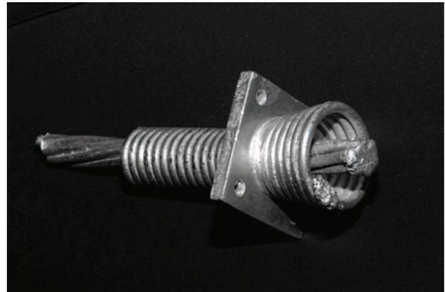
Fig. 2 – Coil Anchorage
